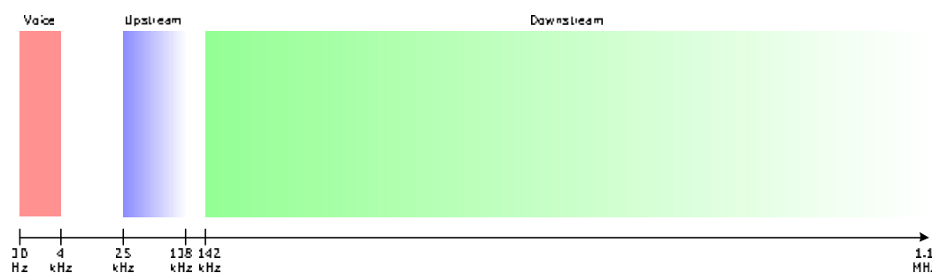
Frequency split for a standard ADSL circuit showing the ranges used for voice, upload and download. Not to scale.
